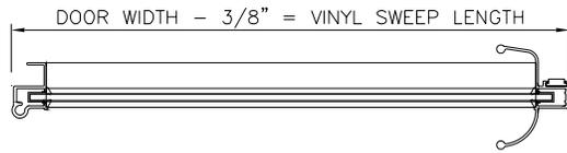
Measure the Door Assembly width, then trim the Vinyl Sweep to 3/8" less than measurement obtained (see figure above).
