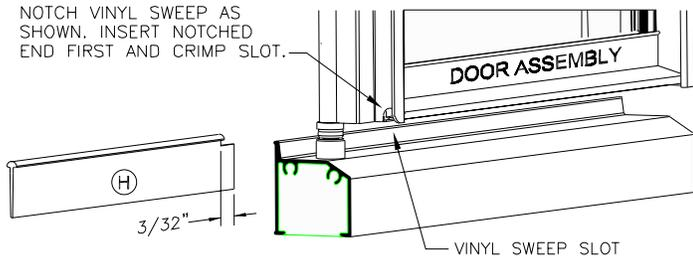
Notch end of Vinyl Sweep as shown. Determine bottom of Door Assembly and insert Vinyl Sweep into bottom rail. Insert 3/32" notched end first.
